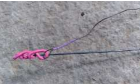
← Tim-N7KOM pulled the clip off the end of a fiberglass pole – a pink hair tie was enough to secure the antenna wire to complete his first HF activation.
