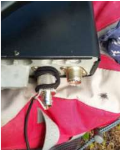
← K7ATN was tugging on the feedline – it was underneath the dog – and the BNC pulled off (shoulda got the dog to move, of course). A hair tie took care of the feedline shield and the center conductor was carefully inserted – activation successful!
