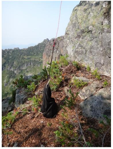
Tall trees are found on summits all over the Pacific Northwest. These make excellent antenna supports for wire antennas of all flavors. I've used an end-fed "random wire" for most of my HF activations. On summits with tall trees, I'll save the time of deploying a squid pole and simply throwing the wire up into a tree.
