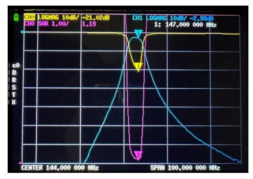
Mike-K6STR was kind enough to run the same test with his NanoVNA. Centering on 144 MHz, with a 100 MHz span. The filter passes through signals from 144 MHz to 148 MHz.
