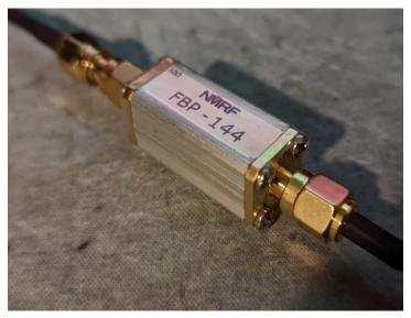
Many summits have high-RF environments from TV or FM radio towers. The front-end filtering on 2m radios can sometimes be overwhelmed by these signals, which completely swamp the receive capabilities of the radio. Chasers may be able to hear an activator transmitting, but the activator won't hear them.
